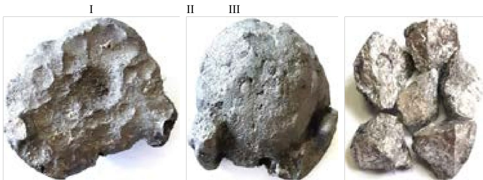
I-II – lump ferroalloy, III – crushed ferroalloy Figure 3 – Photographs of the ferroalloy produced from CAW
